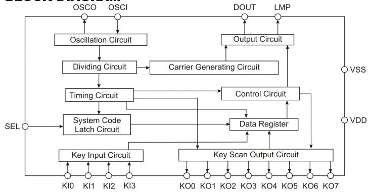
**Infrared Remote Control Transmitter**
