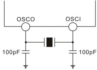
When fosc=455KHz, the oscillation output is divided into 12 parts and the modulation carrier frequency is  $37.9 \sim 39.2$ KHz and 1/3 duty. The 455KHz oscillation is divided into 256 parts and the system fundamental clock is 1.78KHz. The inter-relation between modulation carrier (fc) and the system clock (Tm) with respect to the oscillation frequency (fosc) is given in the equations below.
