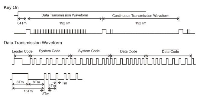
Note: System Clock: Tm = 256/fosc = 0.56ms (at 455KHz)
